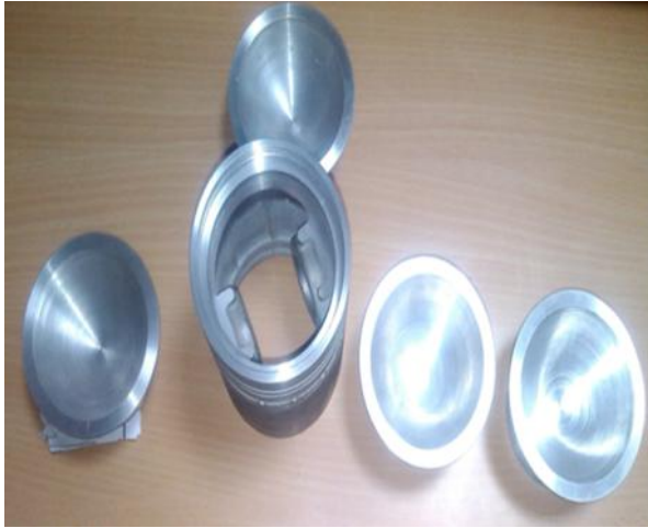
Figure 5. Two piece piston design – base piston and 4 piston crown inserts with squish area of 25%, 30%, 35% and 40%
