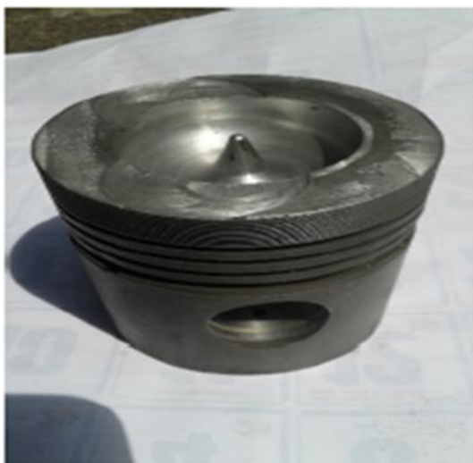
Figure 3. Toroidal CC combustion chamber
